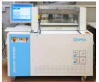
Parametric in-circuit test (fixture)
